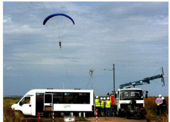
Figure 4: Crosswind device with ground-based generation. Image: KPS
