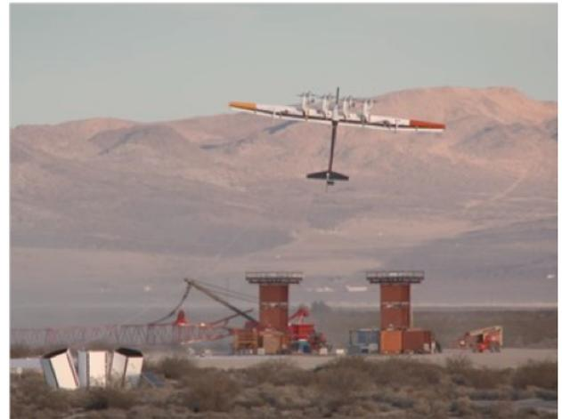
Figure 3: Crosswind device with on-board generation. Image: Makani
