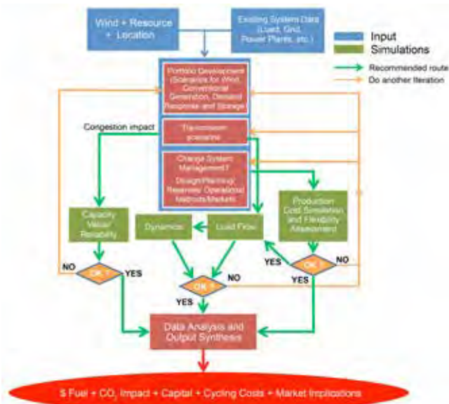
Figure 2. Flow chart of a complete wind integration study, showing relevant iteration loops from simulations to set-up and portfolio development
