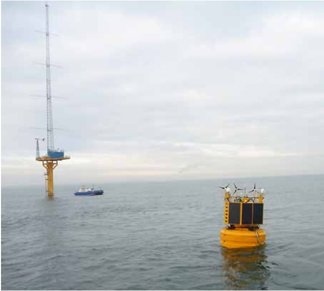
Figure 5. FLiDAR floating lidar system (Source: www.leosphere.com/products/floating/flidar-floating-buoy-lidar )
