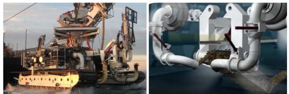
Figure 7: (left) typical hard ground mechanical trencher, which needs to be heavy (normally more than 40t in water); (right) trench being formed by the cutting chain. Both images courtesy of Helix Canyon Offshore.
