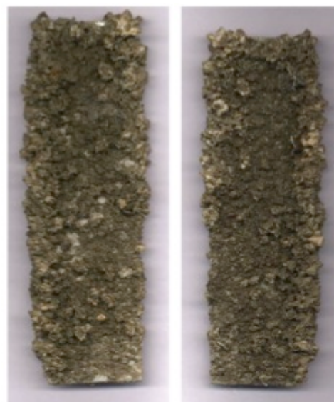
Figure. 4b. Barnacle Growth on X2CrNi18-9 Stainless Steel Plate after 224 Days Immersion in Sea Water.
