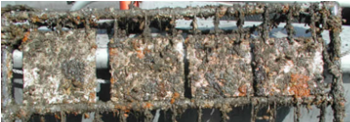
Figure. 2a. Hard Biofouling Community Developed on steel plates over 1 year. Bridger Scientific, 2005
