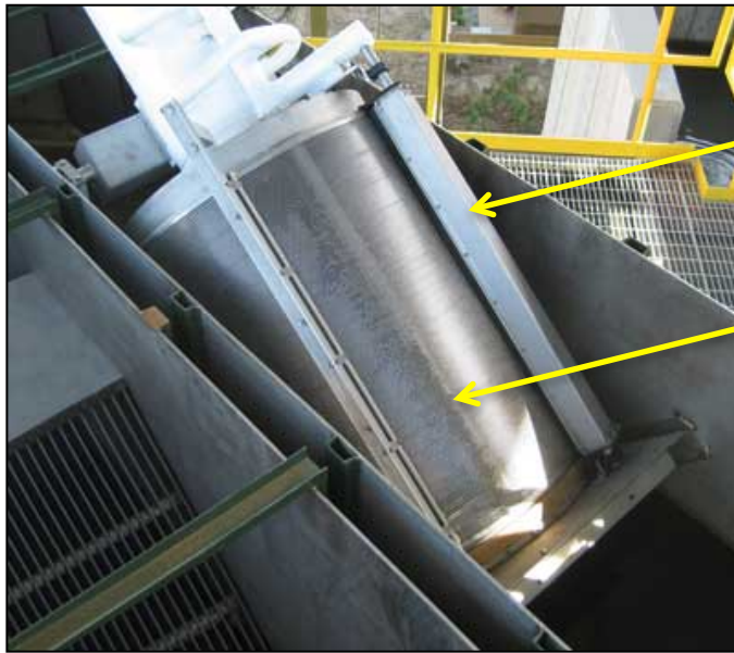
Figure 11a. A Self-Cleaning Rotating Drum Filter at a Fish Farm Water Inlet. Waterworld, 2014
