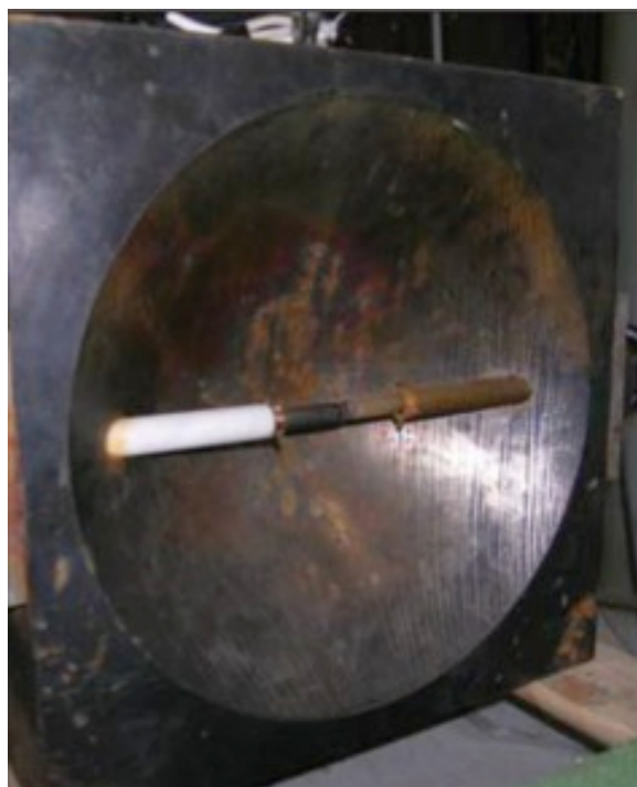
Figure 17b. Two electrodes of a pressure pulse device inside a directional reflector.
