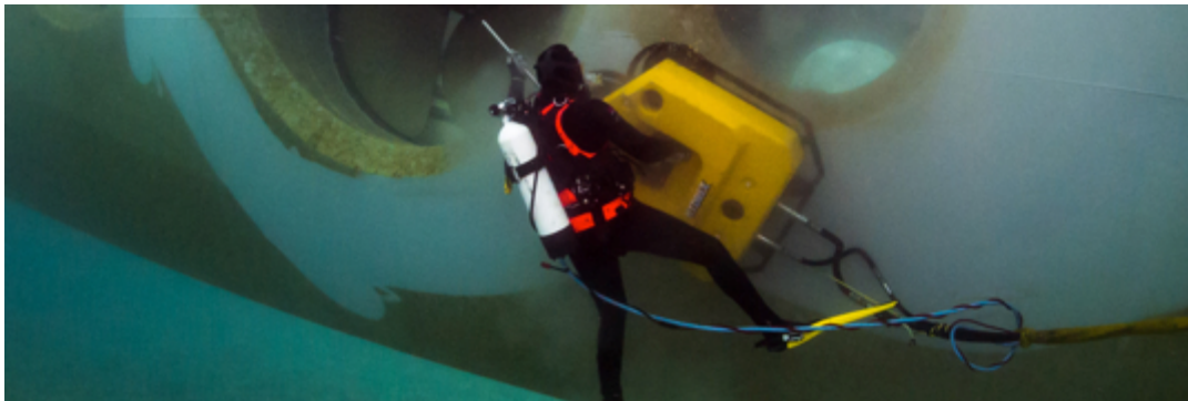
Figure 11b. A Diver Removing a Slime Layer from a Hull. Hydrex, 2011
