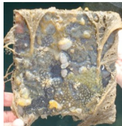
Figure. 2b. Soft Biofouling Community Developed on a Polystyrene Sheet Submerged in a Scottish Marina for 8 Weeks. Marine Scotland, 2014
