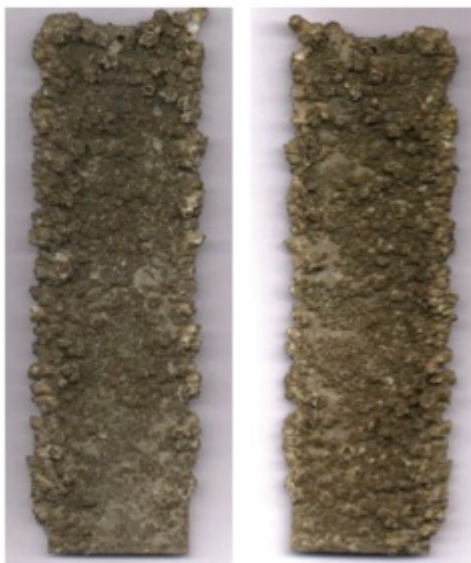
Figure. 4a. Barnacle Growth on Grade 2 Pure Titanium Plate after 224 Days Immersion in Sea Water.
