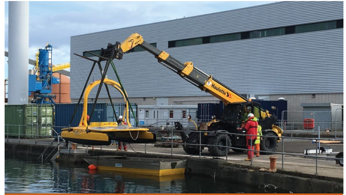
The ASV being deployed into the dock, with remote crane access alongside the dock area
