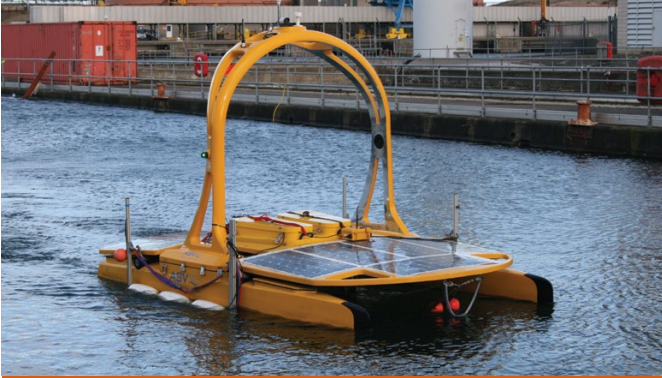
The BioSonar technology detecting cables buried in the seabed of the saltwater dock facility
