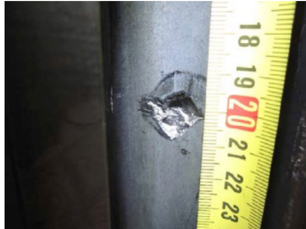
Figure 7: Ring gear (first stage): severe indentation
