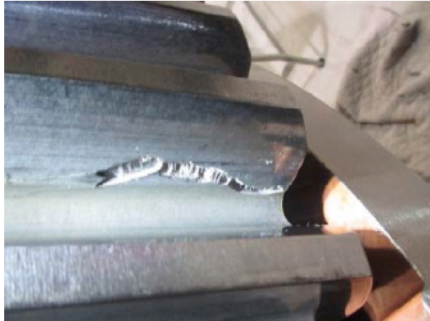
Figure 6: Planet gear 3. Flank of sun pinion mesh. Fractured tooth. Rotor side end.
