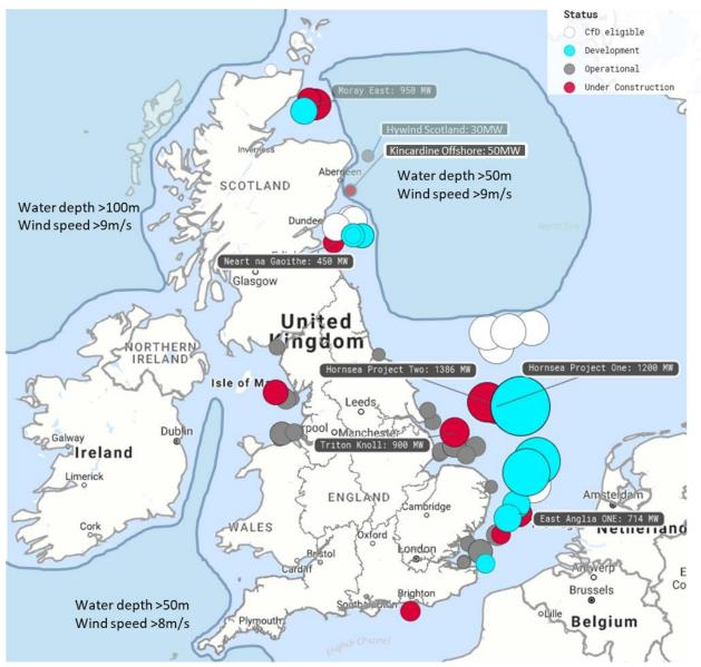
Figure 1: Indicative floating wind locations compared to existing UK offshore portfolio (Sources: DNV-GL, 2014 via Carbon Trust, Floating Offshore Wind: Market and Technology Review 2015; and ORE Catapult mapping via Espatial.com)
