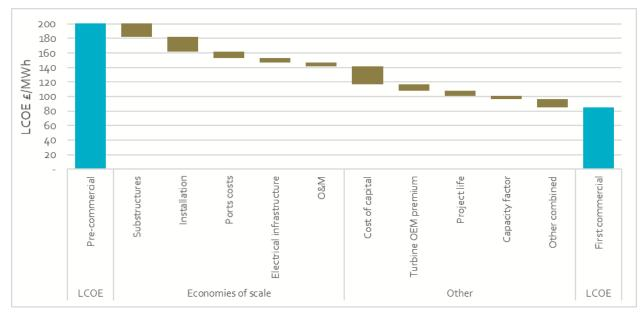
Figure 2: Floating wind cost reduction drivers from Pre-commercial to First Commercial Projects
