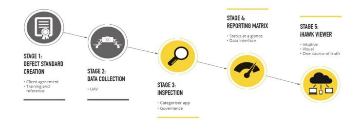
Figure 2: Cyberhawk's UAV inspection campaign process
