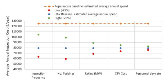
Figure 7: Sensitivity of UAV inspection cost to O&M cost model input values
