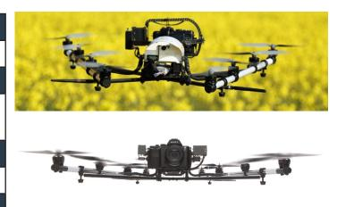
Figure 6: Sony  $\alpha$ 7 mounted to a Falcon 8
