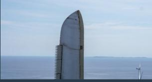
In late 2017 Cyberhawk was tasked by Siemens Gamesa to carry out visual inspections of 27 wind turbines at an offshore wind farm <sup>[3]</sup>. Unique to this inspection campaign was the requirement to develop a bespoke app to meet specified requirements: a 25% overlap in images to ensure no blade surface was missed. In this case the images of each individual turbine were processed and uploaded on the same day as inspection.
