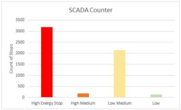
Figure 2: Alarm count of automatically-defined stop groupings.
