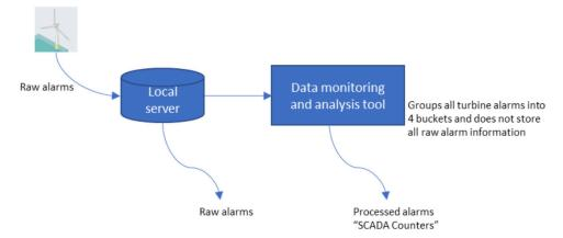
Figure 1: Turbine alarms being stored locally and being processed by a data monitoring tool.
