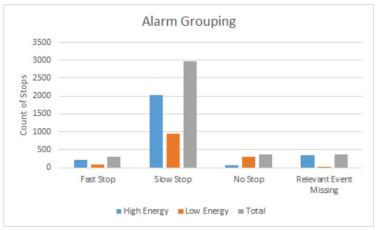
Figure 3: Alarm count of internally-defined stop groupings.
