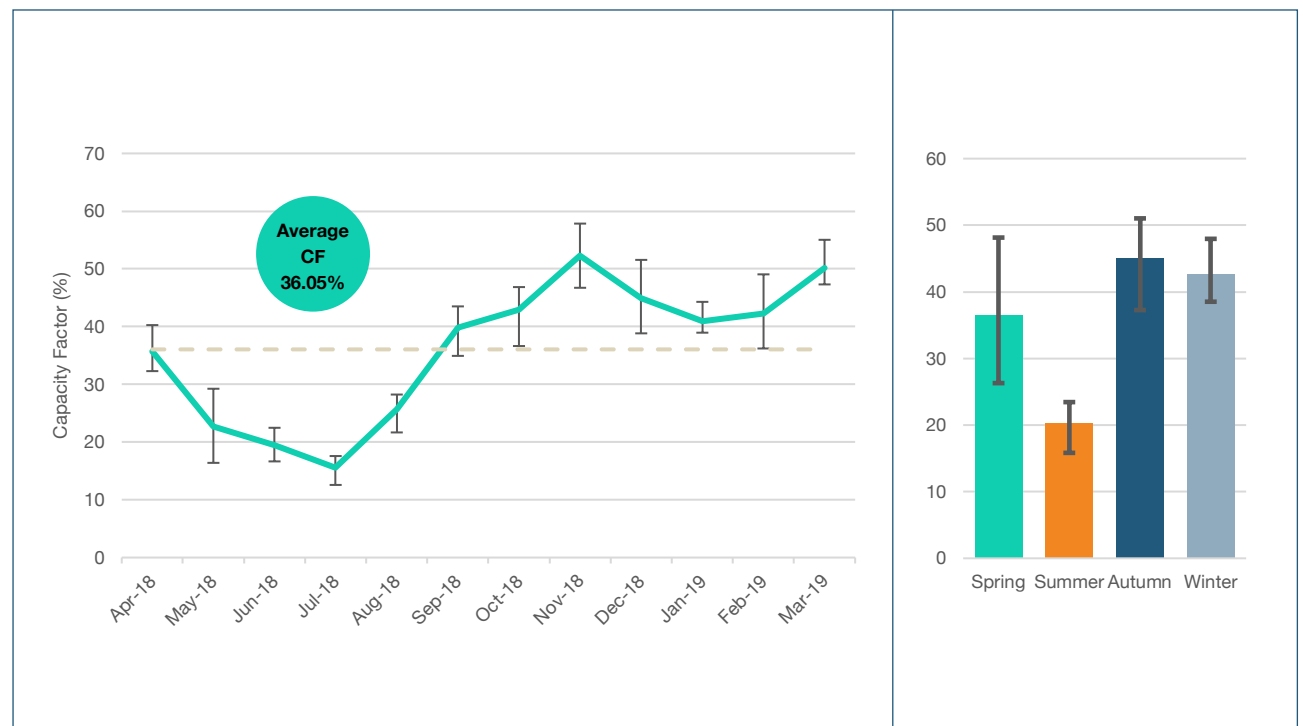
Figure 4 - Average Capacity Factor Over Year, Right Showing Seasonal Averages (error bars represent P25 & P75)
