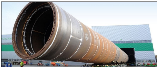
Figure 2: Monopile (source: Boskalis)
