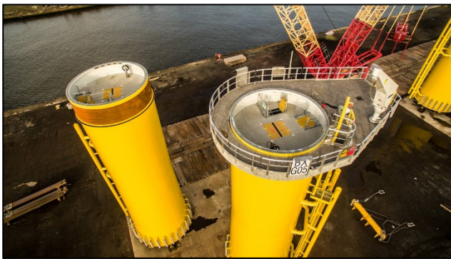
Figure 3: Transition pieces (source: EEW)
