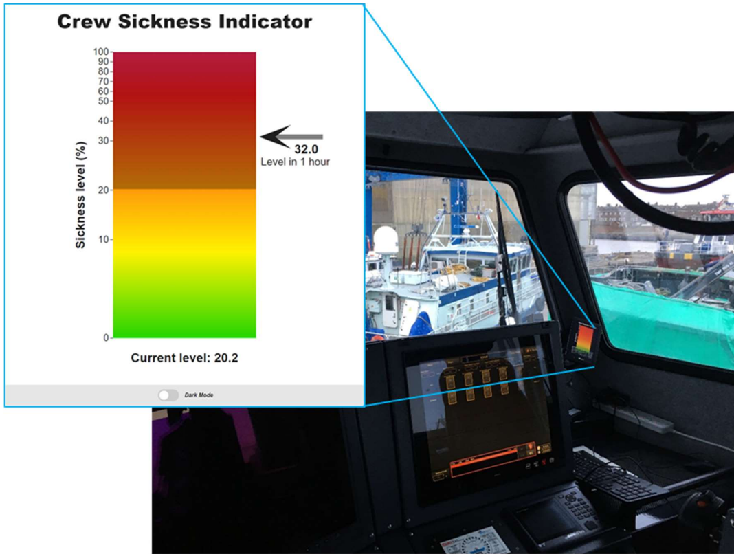
Figure 6: MSI indicator installed onboard a CTV bridge
