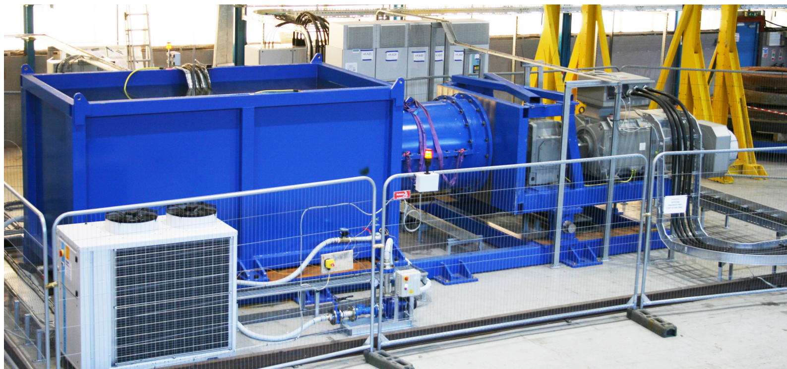
image above 1MW Powertrain test rig
