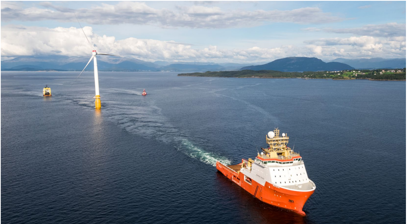
Hywind Scotland turbine being towed into position. (Credit: Equinor)
