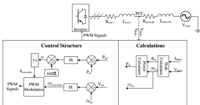
Figure 2: Simple representation of a power converter controlled as VSM connected to the grid
