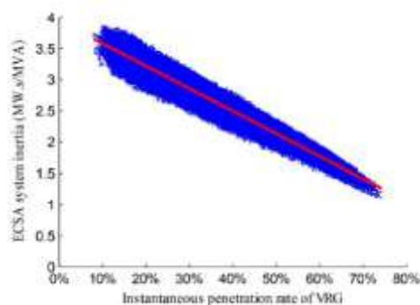
Figure 1: The relation between renewable energy penetration and inertia [2]
