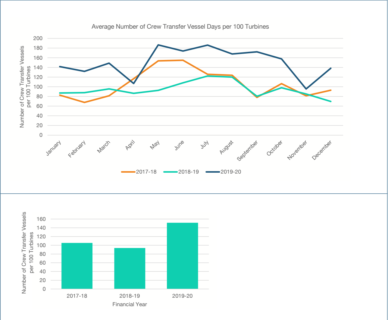
Figure 17 - Number of Crew Transfer Vessel Days per 100 Turbines Trends (top = monthly values, bottom = yearly values)
