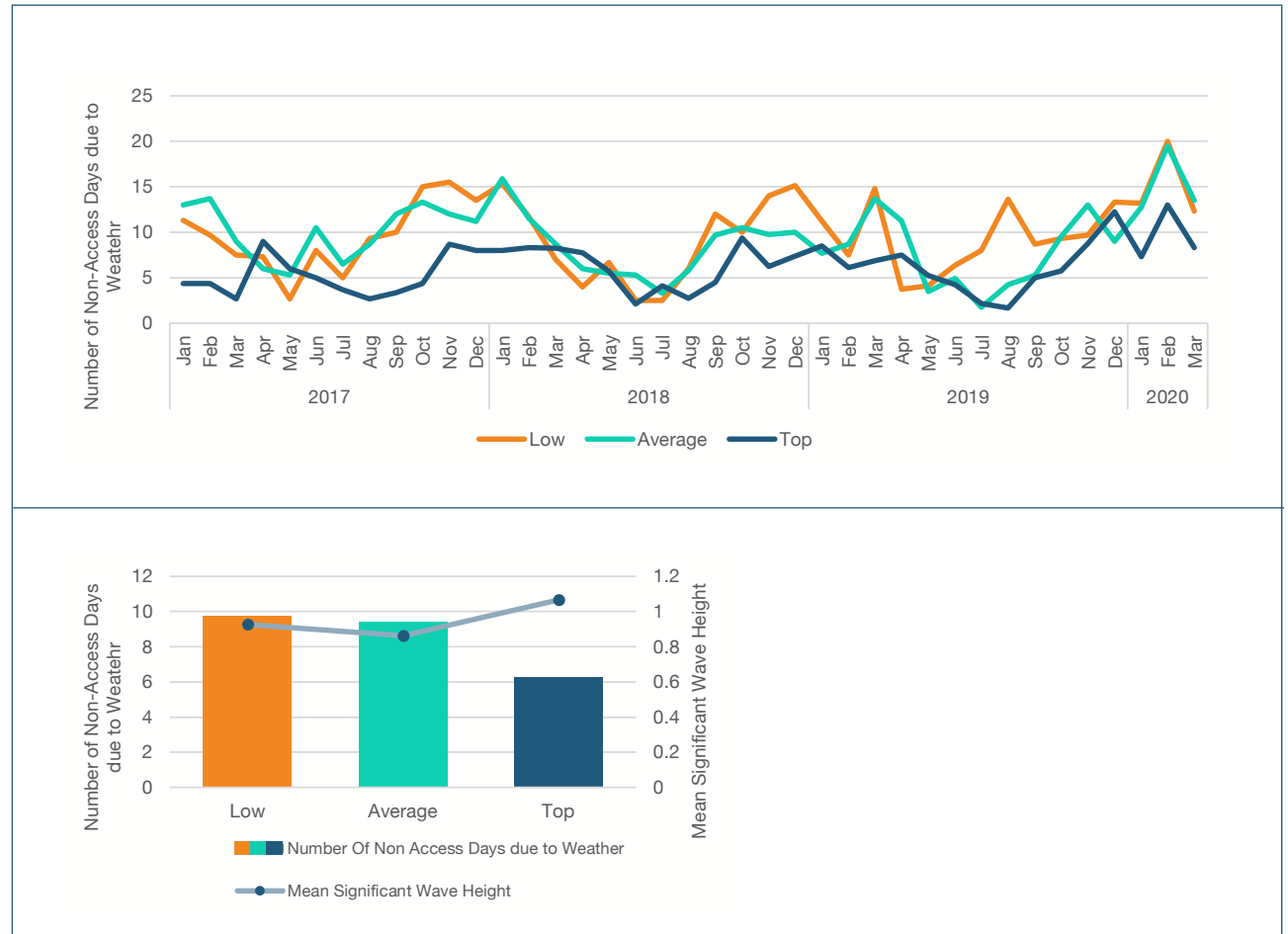
Figure 24 - Top = Number of non-access days split by performance group (Jan 2017 - Mar 2020) Bottom = Average number of non-access days and significant wave height (Jan 2017 - Mar 2020)
