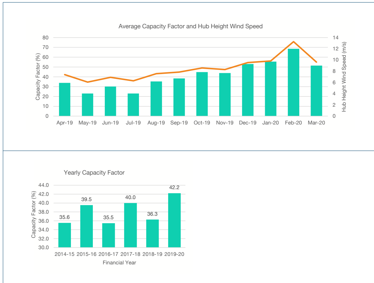
Figure 5 - Capacity Factor Trends (top = 2018-2019 monthly with average wind speed shown, bottom = yearly average)
