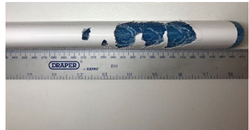
Figure 1 - Example of severe erosion in an accelerated environment
