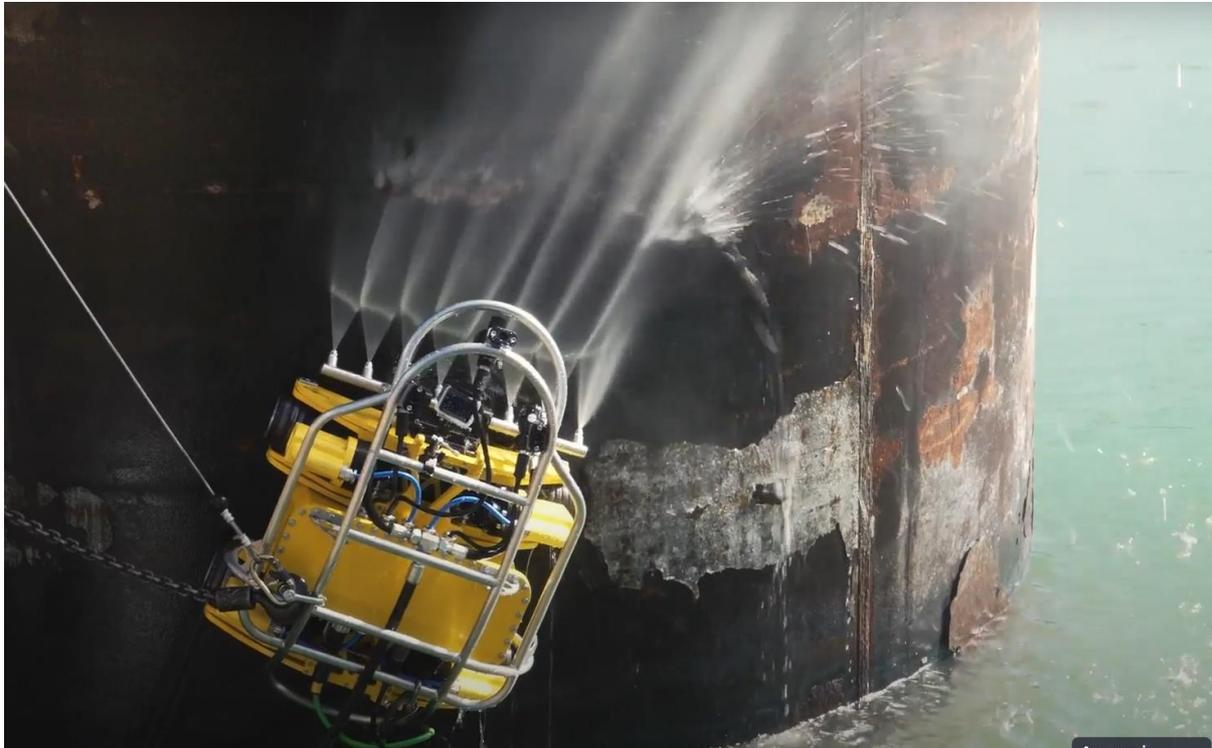
*IMAGE 1. Innvotek’s Amphibian demonstrates its inspection and cleaning capabilities at ORE Catapult’s National Renewable Energy Centre in Blyth, Northumberland. This platform has a variety of applications in the wind, shipping and oil and gas sectors.*
