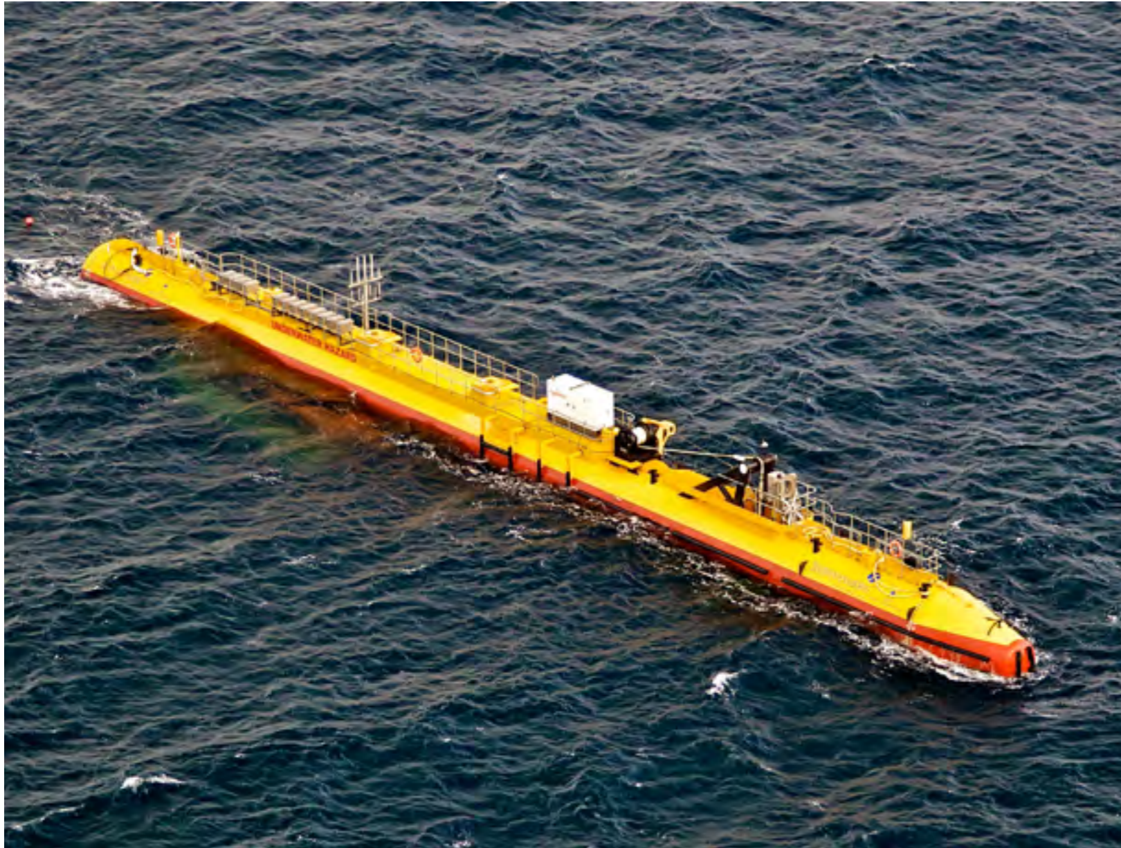
SR2000 testing at EMEC's Fall of Warness test site (Image courtesy of Orbital Marine Power)
