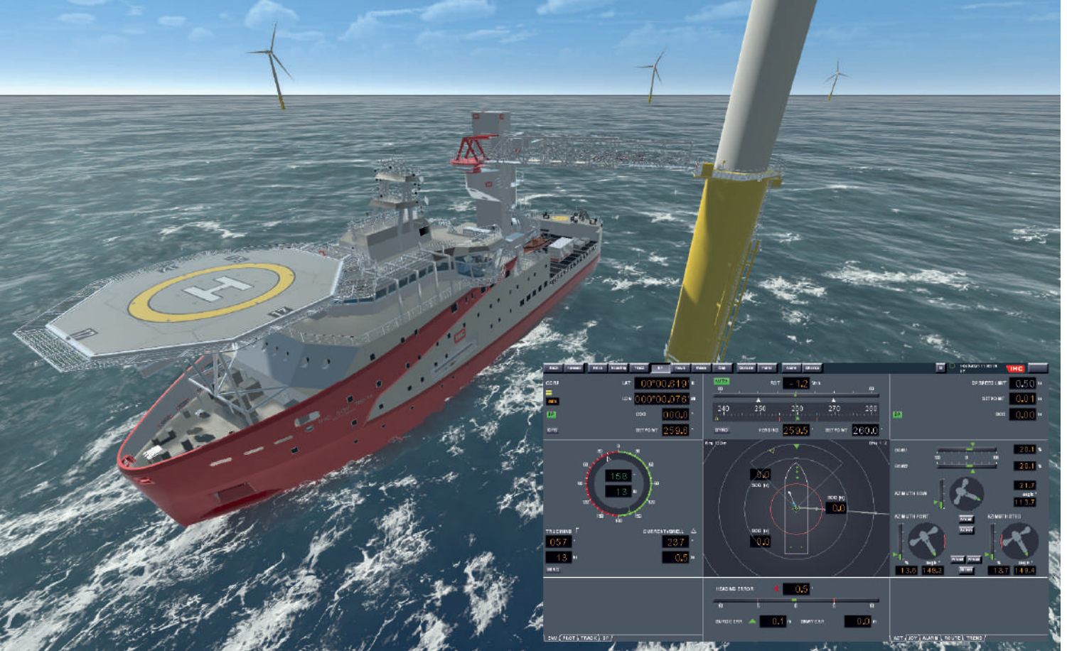
Figure 23. The simulator environment, showing the 3D viewer with the Royal IHC DP system overlay. (Source: Royal IHC)
