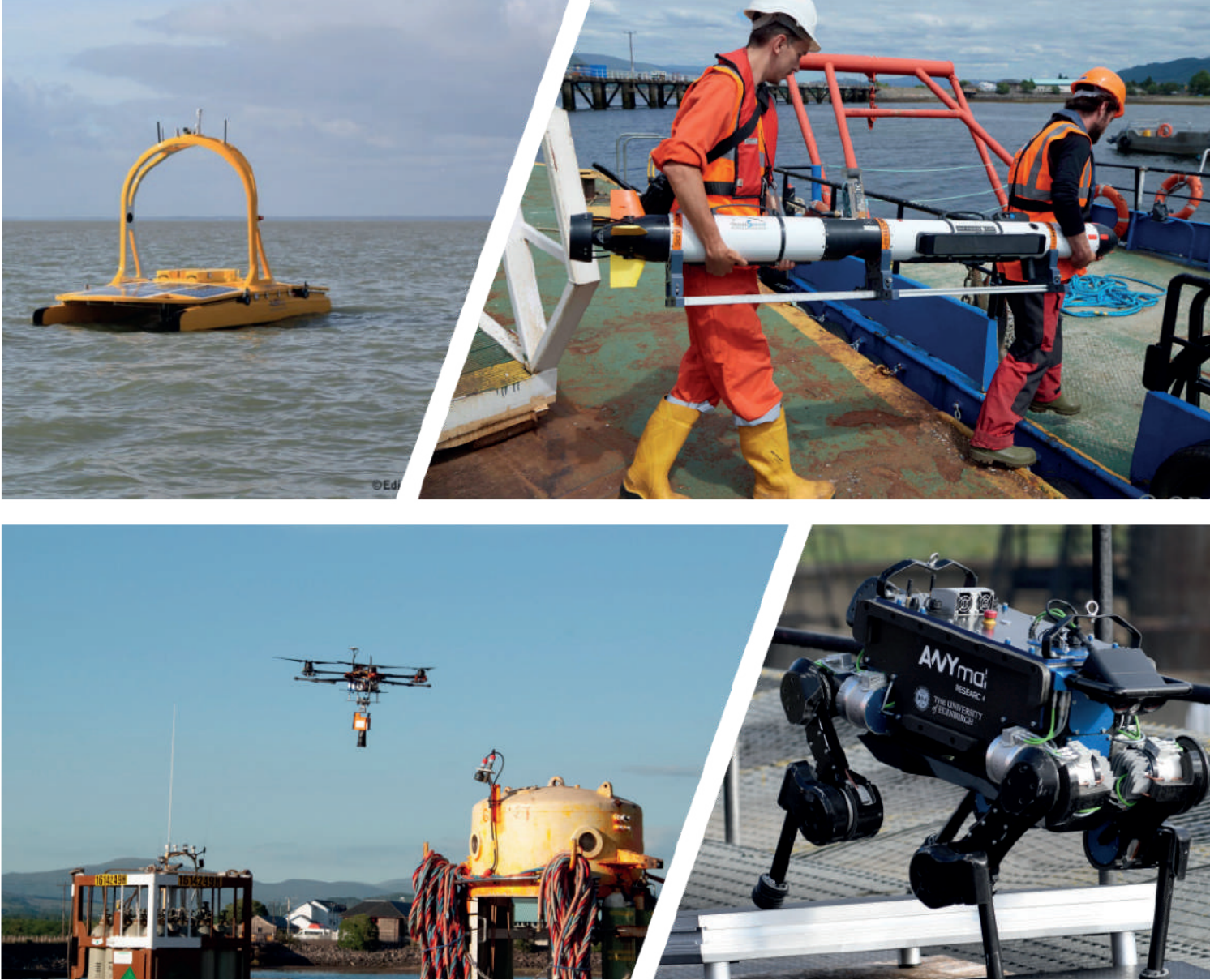
Figure 5. Surface, subsea, ground and aerial robots for offshore environments. (Source: ORCA Hub.)
