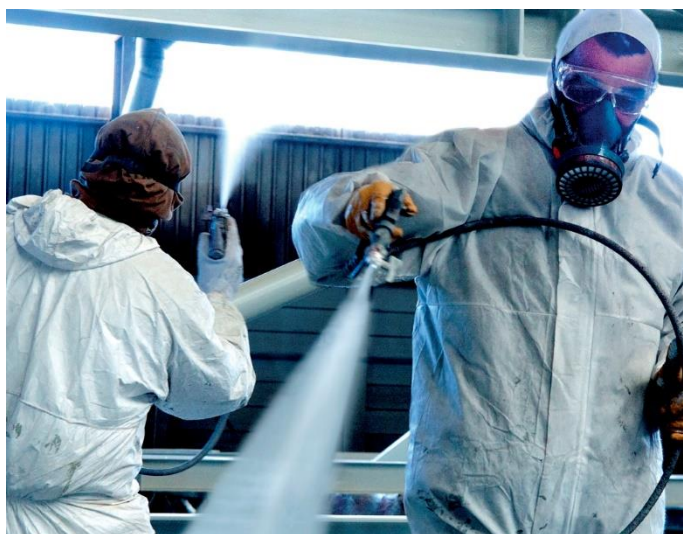
Figure 20: Hempel spray painting process. Power and Cables. (2022). Wind Turbine Tower . https://www.powerandcables.com/cable-cleats-wind-energy/wind-turbine-tower/
