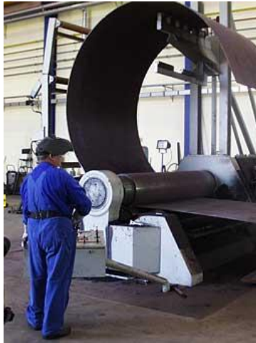
Figure 21: The rolling process for manufacturing a steel conical tubular tower.[25]
