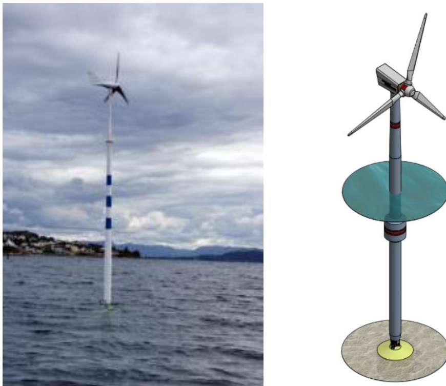
Figure 15: Left: the scale model currently in deployment. Right: A 3D model of the full-scale concept design. [19]
