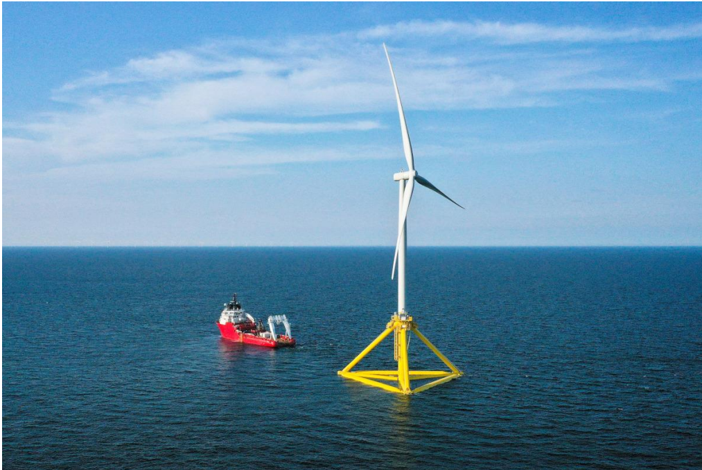
Figure 8: TetraSpar being towed to its new location. [9]
