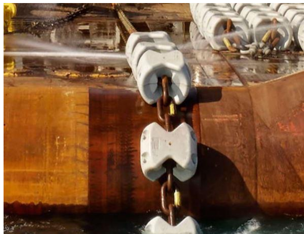
Figure 14: Clump Weights Being Deployed [20]
