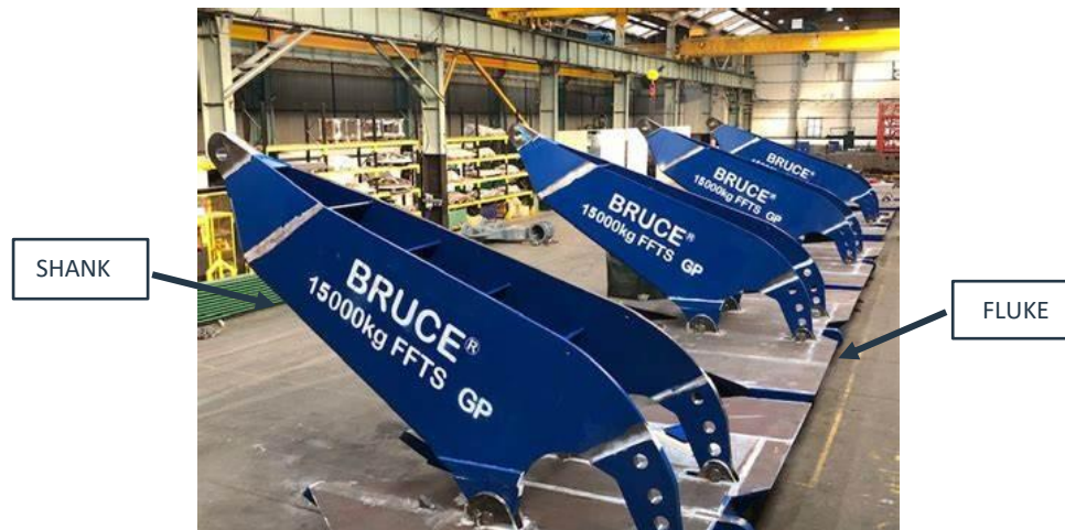
Figure 12: Anchor Production Line [18]
