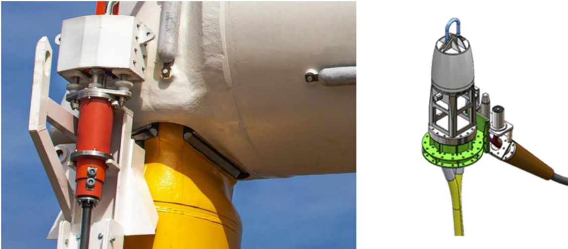
Figure 19 - Left: Nova Innovation's NovaCan connector [87]. Right: Quoceant Q-Connect connector [88].
