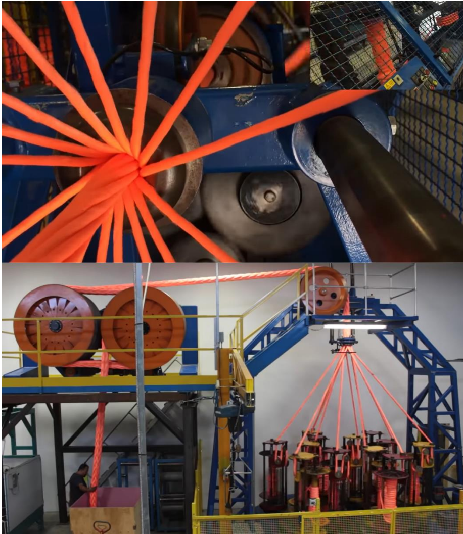
Figure 15 - Machinery used to manufacture Dyneema synthetic rope. Top: Multiple strands of rope are brought together using a stranding machine to manufacture the synthetic rope sections. Bottom: An example of a braiding maypole machine, used to braid the rope sections together into the final product. Source: Atlantic Braids Ltd, Youtube ( https://www.youtube.com/watch?v=ndmXL-ygqdM&t=201s , accessed 05/05/22)
