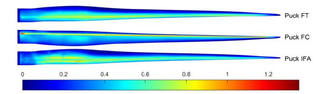
**Pictured:** Contour plot of the Puck failure criterion for a redesign of the blade for the IEA 15MW reference turbine. A value of 1 indicates that the material has failed, so this preliminary design shows good material utilisation without major failures. Compared to the original design this blade is 4% longer, reduces blade mass by 11%, increases AEP by 1.5% and reduces LCoE by 2.3%
