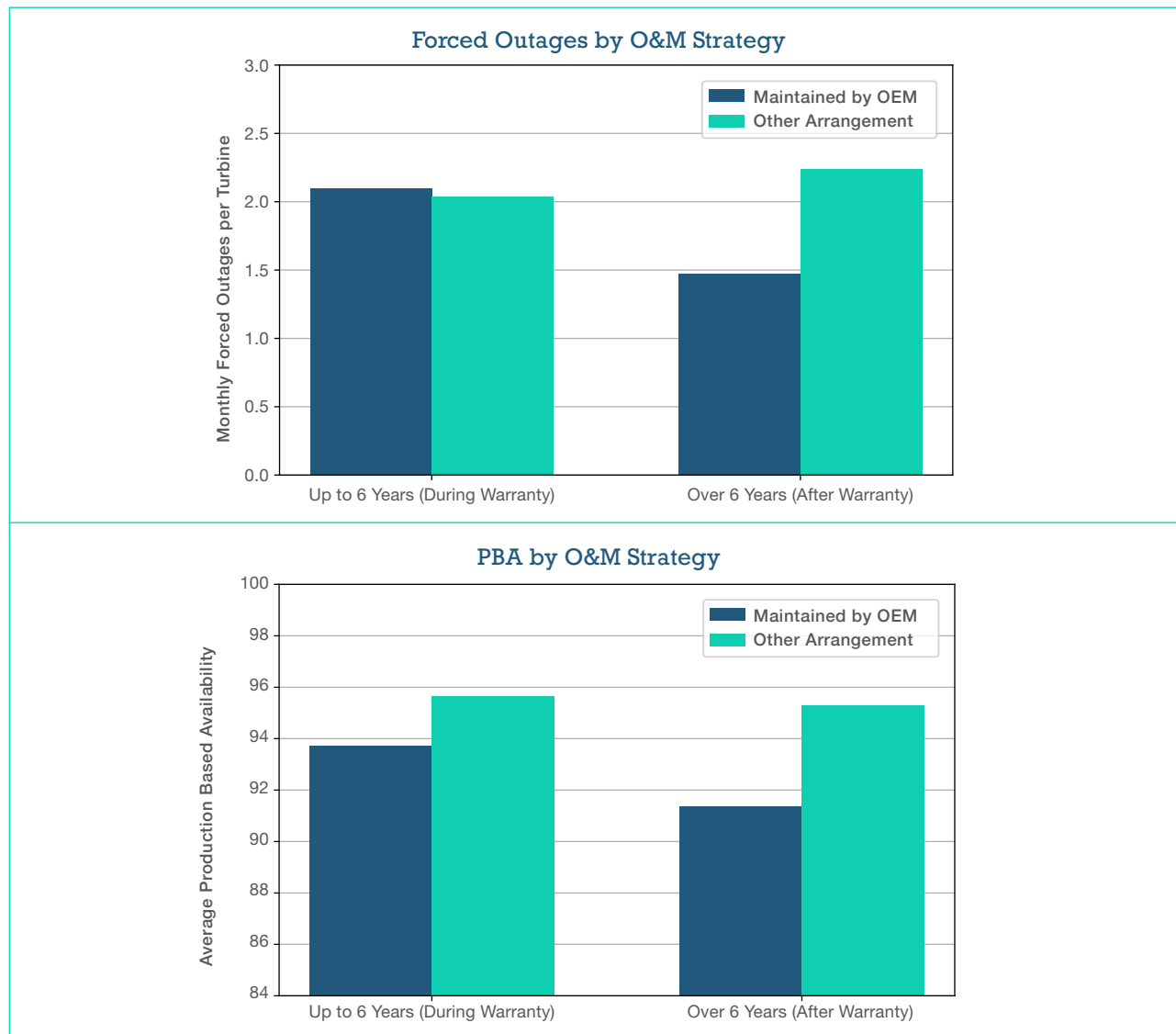
Figure 17 Average number of monthly forced outages per turbine by O&M strategy before and after typical warranty period (6 years) (top) and corresponding average of PBA (bottom).
