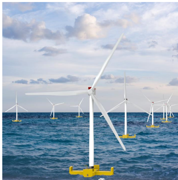
Figure 2: VoltornUS+ Hull Technology (image credits University of Maine)
